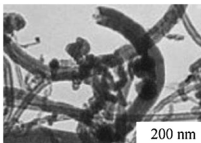
(c) No.3-CNT, L=1.5\mu m , d=80nm
